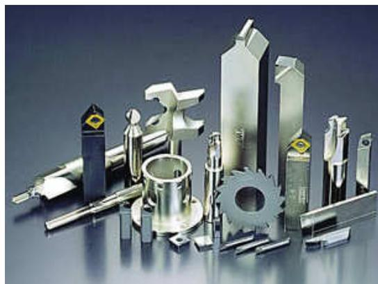
Figure 1. Polycrystalline diamond cutting tools
