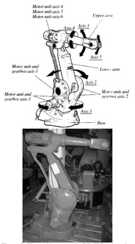
Figure 7. The architecture of ABB-IRB type robot
