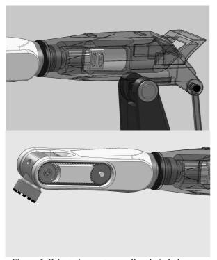
Figure 6. Orientation system: roll and pitch degrees
