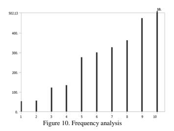
The diagram of frequencies is presented in table (2). This reveals that the first natural frequency of 51.8 Hz, which confirm a fair parameter of stiffness and a low probability to get into a resonant frequency during the execution.
