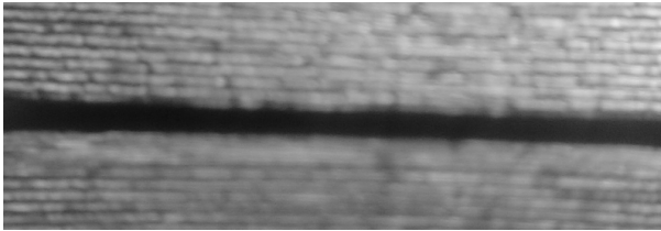
Figure 6. The processed surface after turning with cutting feed f=0.083 mm/rot, step 4
