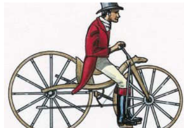
Figura 3. Drezină cu antrenarea roții spate prin mecanism cu bare articulate Figure 3. Draisienne with rear wheel driving through hinged-rail mechanism
