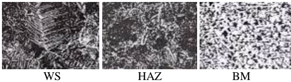
Figure 8. Metallographic structure of manually welded seam with coated electrode, the pipe \Phi 108 \times 4 OLT 45 (240:1)
