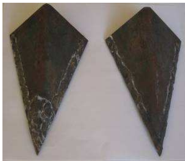
Figure 8. Welded hardfacing plough
