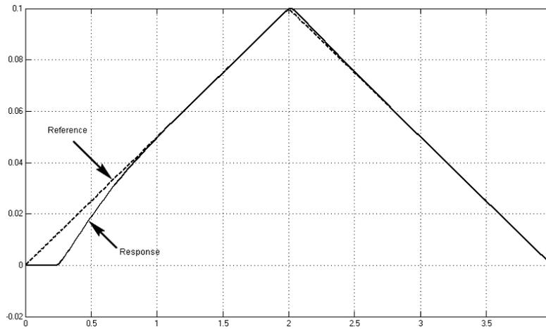
Figure 3. Triangular reference and the response of the controlled system (100 N constant perturbation)
