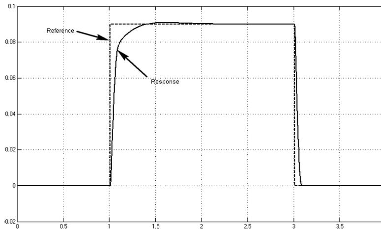
Figure 4. Pulse reference and the response of the controlled system (100 N constant perturbation)
