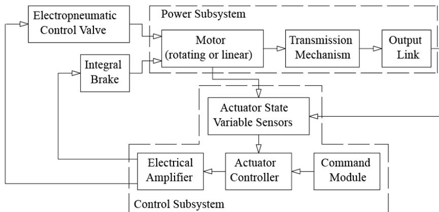
Figure 1. Block diagram of the pneumatic actuating system [1]
