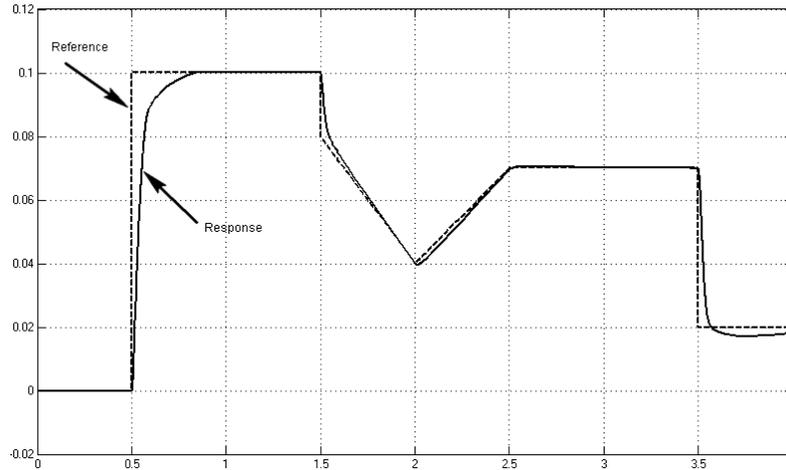
Figure 5. Variable reference and the response of the controlled system (100 N constant perturbation)
