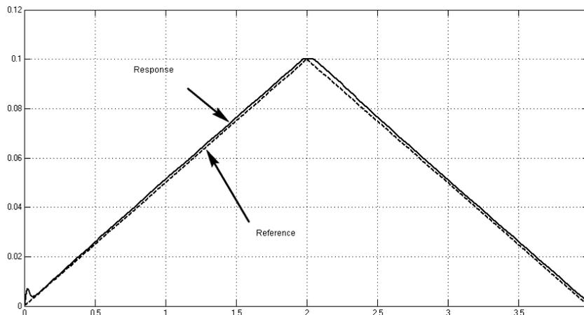
Figure 6. Triangular reference and the response of the controlled system (linear variable 0 - 100 N perturbation)
