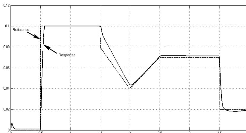
Figure 8. Variable reference and the response of the controlled system (linear variable 0 - 100 N perturbation)
