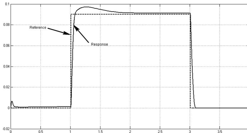
Figure 7. Pulse reference and the response of the controlled system (linear variable 0 - 100 N perturbation)
