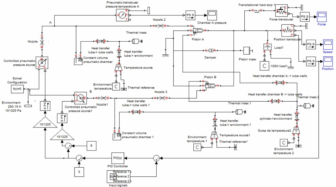
Figure 2. Pneumatic system double acting cylinder with PID controller
