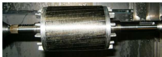
Figure 2. Shaft mounted before machining
