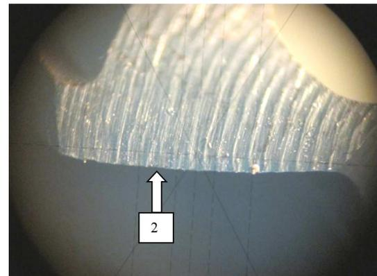
Fig. 5. Cutting lip Tp1 (1), Tp2 (2), chisel edge  $T_t$  (3) and corner (4) for drill no. 4 from Table 2
