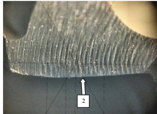
Fig. 4. Cutting lip Tp1 (1), Tp2 (2), chisel edge  $T_t$  (3) and corner (4) for drill no. 1 from Table 2
