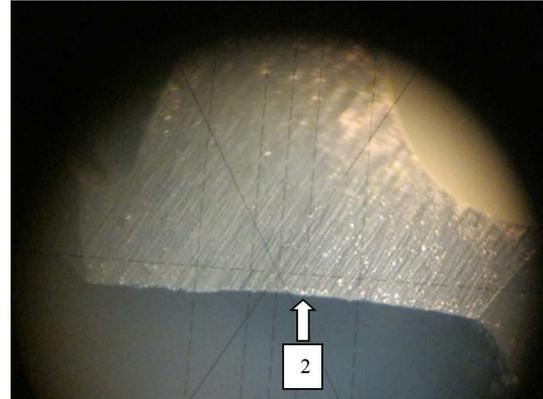
Fig. 3. Cutting lip Tp1 (1), Tp2 (2), chisel edge  $T_t$  (3) and corner (4) for drill no.3 from Table 1
