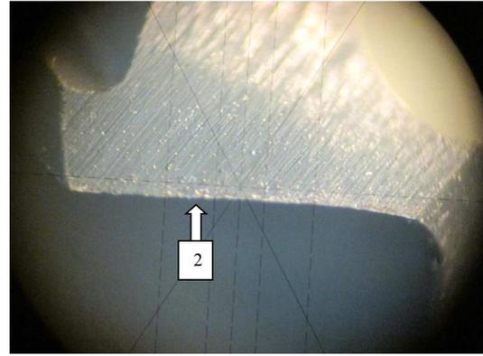
Fig. 2. Cutting lip Tp1 (1), Tp2 (2), chisel edge  $T_t$  (3) and corner (4) for drill no. 1 from Table 1
