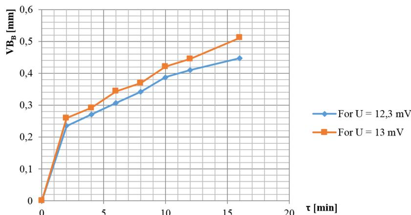
Fig. 1. Graphical representation for tries at wear (processed after [2])
