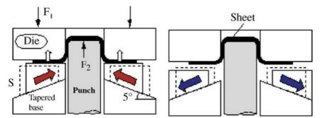
Fig. 2. Deep drawing using tapered blank holder divided into for segments [6]
