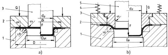
Fig. 1. Deep drawing dies with: a) - plane blank holding; b) – combined blank holding
