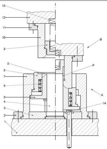
Fig. 3. Combined blank holding deep drawing die
