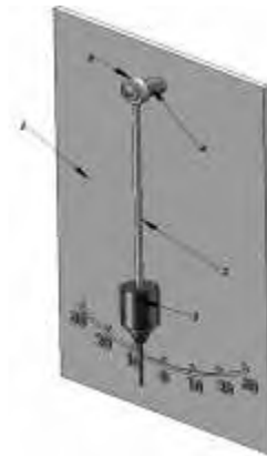
Figure 2. 3D model of the experimental setting 1 – base; 2 – pendulum; 3 – weight; 4 – lease; 5 – bearing bush
