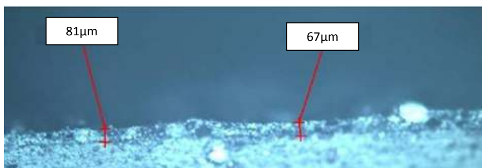
Figura 4. Imagine la microscop a stratului de TPE glisant Figure 4. Microscope image of sliding TPE layer
