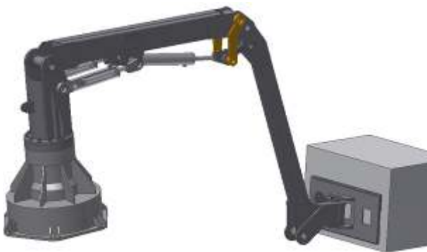
Figure 2. 3D CAD model of hydraulically driven manipulator
