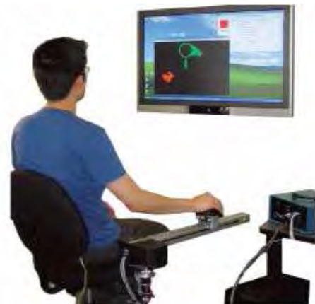
Figure 2. Quanser Autonomous Upper-Limb Stroke Rehabilitation Device [5]
