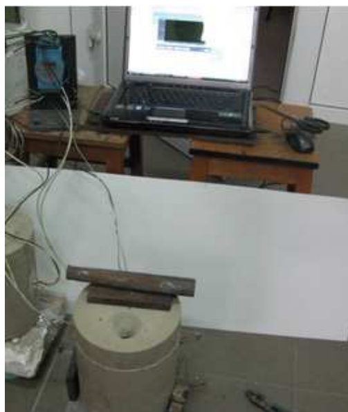
c) The equipment to temperature measuring and recording
