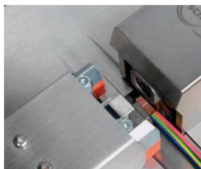
Fig. 4. View of wires placed in the welding machine
