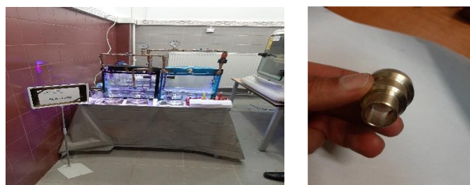
Fig. 5. Filtration installation type SCA-1700 and CWF filter mounting bracket
