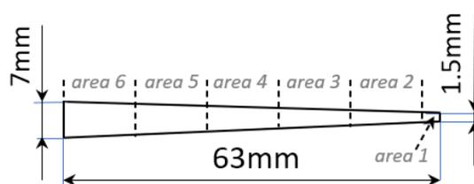
Fig. 1. Wedge-shaped sample and splitted areas for evaluation
