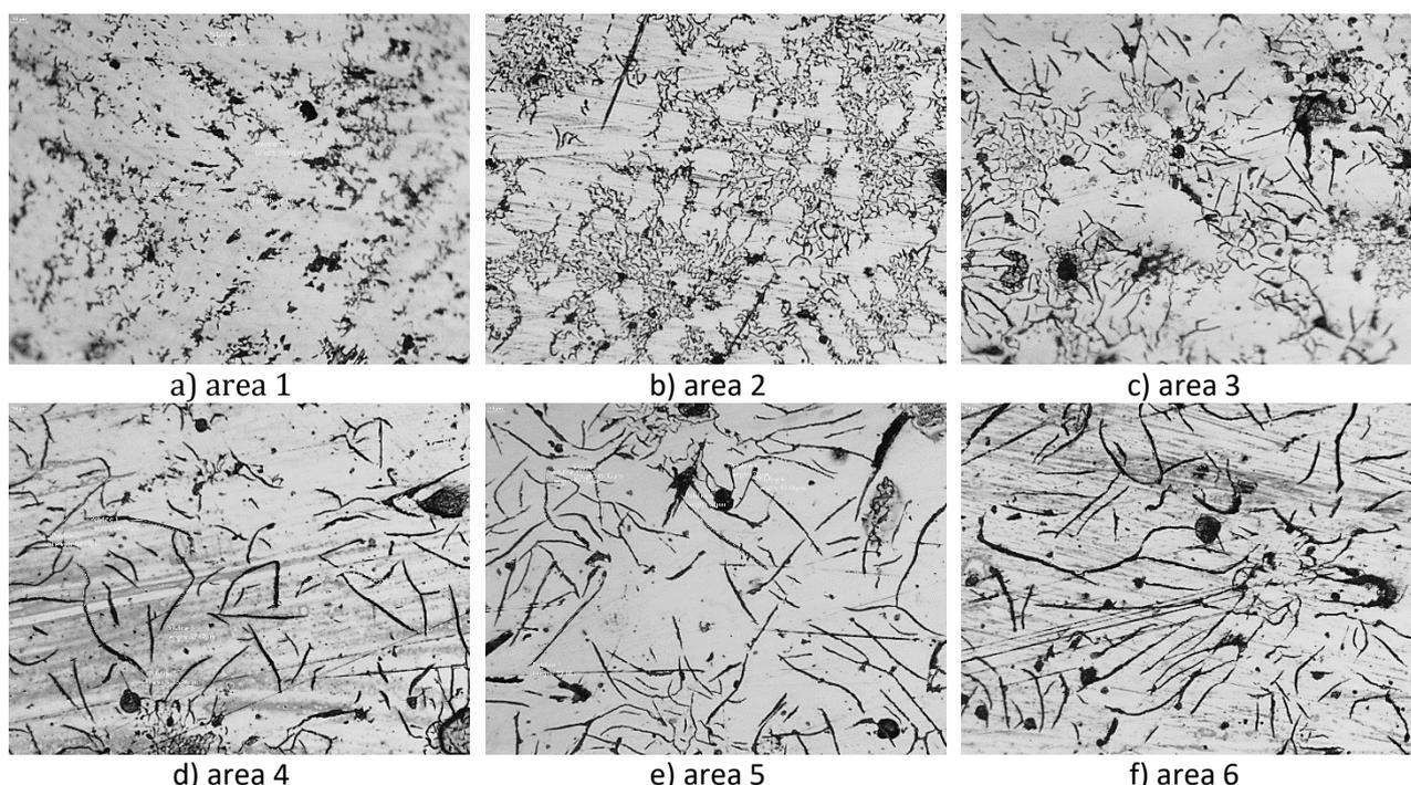
Fig. 2. Microstructures of gray cast iron sample used for graphite size evaluation (X200)
