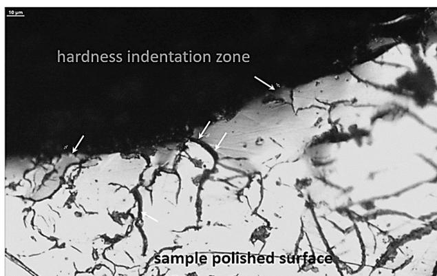
Fig. 4. Edge between indentation and polished surface
