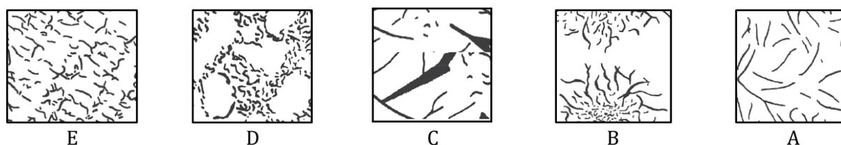
Fig. 3. Distribution forms of graphite flakes (lamellar), from SR EN ISO 945-1
