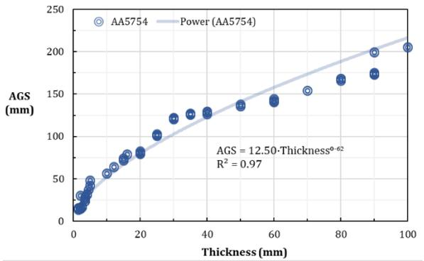
Fig. 9. Relationship between AGS and thickness of AA5754 by using power regression
