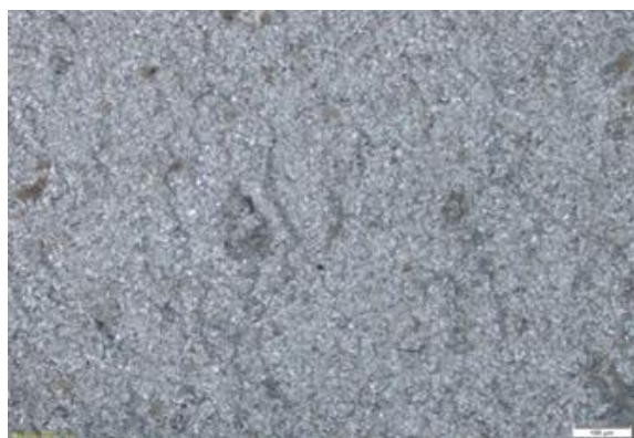
Fig. 3. 40Cr130 hardened at 1040^{\circ}\text{C} , tempered at 510^{\circ}\text{C} held in liquid nitrogen vapours for 30 minutes at -(85-90)^{\circ}\text{C} and fractured at -80^{\circ}\text{C} . Etching reagent: aqua regia. 100:1
