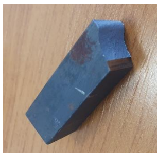
Fig. 1. Specimen three fractured (breaking section) at -80^{\circ}\text{C} after immersion in liquid nitrogen for five minutes, down to -196^{\circ}\text{C}
