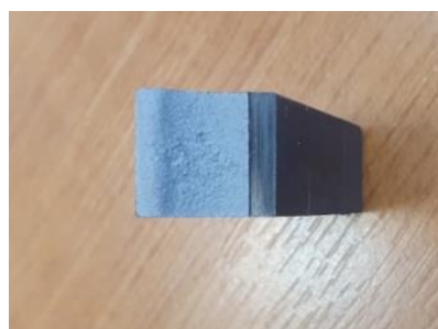
Fig. 2. Specimen four fractured (breaking section) at -80^{\circ}\text{C} immersed in liquid nitrogen, for 30 minutes, down to -196^{\circ}\text{C}
