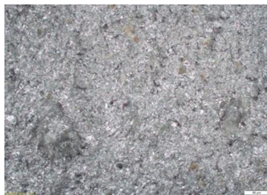
Fig. 4. 40Cr130 hardened at 1040^{\circ}\text{C} , tempered at 510^{\circ}\text{C} held in liquid nitrogen vapours for 30 minutes at -(85-90)^{\circ}\text{C} and fractured at -80^{\circ}\text{C} . Structure: martensite + carbides. Etching reagent: aqua regia. 500:1
